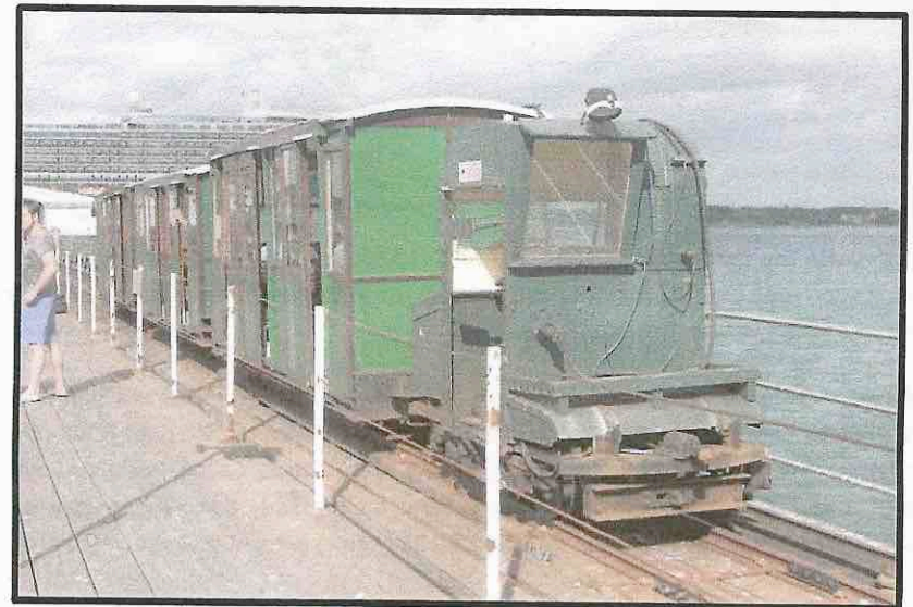
This picture shows the 1909 Hythe Pier Tramway, electrified after WW1, and is still running. The loco is the original, but over time the coaches have been updated. Alan Henshall sent this photograph in, after using a ferry from Red Funnel terminal to the Hythe Pier.
