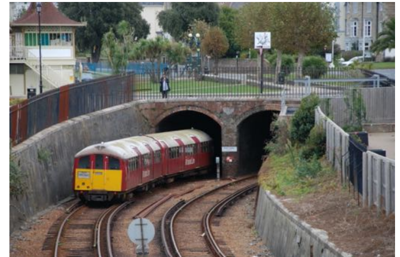
Unit No. 483008 takes the Down line through the twin tunnel's under Ryde Esplanade with a train for Shanklin. This shows the limited clearances and why main line stock cannot be used on the island.
