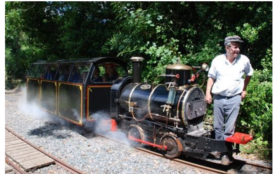
The driver stands just above rail level in this push-pull operation. The train is about to leave Mines Yard for Valley Gardens on 24 th June 2023, Note the seat at the front so the driver can sit down through the tunnel section.
