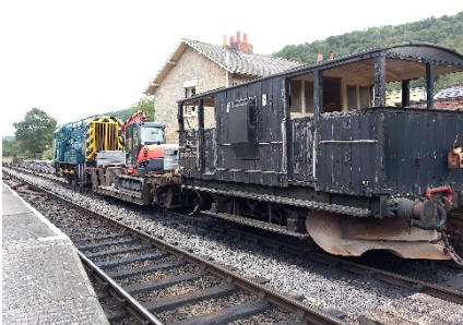
A BR 20 tonne Shark brake van pictured stabled in the loop at Levisham on the North Yorkshire Moors Railway.
